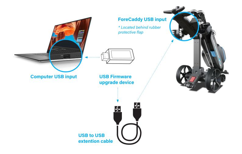
**Note:** Firmware upgrade 5.0 requires you to use the USB Firmware upgrade device and connect it to your ForeCaddy via the USB to USB extention cable. Firmware upgrade 5.0 does not require you to upgrade the remote control.
