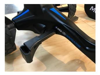
1. To insert the horizontal seat stem ensure the coloured leaver underneath the chassis is unlocked as per the below image
