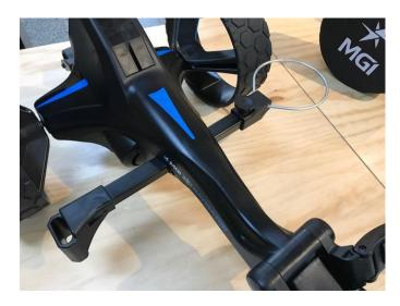
7. Fit the sand bottle adaptor onto the left hand side of the seat stem and fasten the screw until firm
