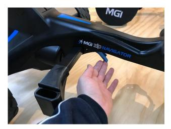
4. You can now fit the seat onto the horizontal seat stem
