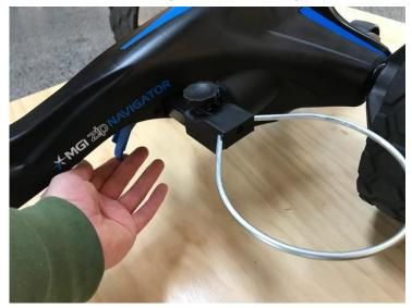
11. If you are fitting a sand bottle only, release the coloured lever underneath the buggy and insert the sand bottle adaptor through the centre of the chassis
