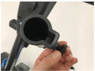
8. Insert the umbrella holder extender into the umbrella holder and fasten the block against the umbrella holder extender until firm and secure.
