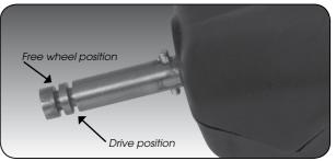
*i. Drive position* – Lock the wheel onto the groove closest to the battery base. To do this, press the grey release button on the wheel hub, push the wheel on to the axle as far as possible. To test for drive position try rolling the wheel backwards. If you feel resistance then the wheel is now in drive position and ready to use. Repeat for both wheels.
